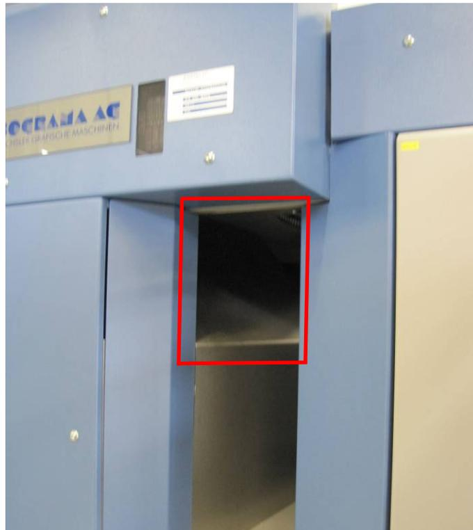
Figure 4: Hazard point, rejector chute
