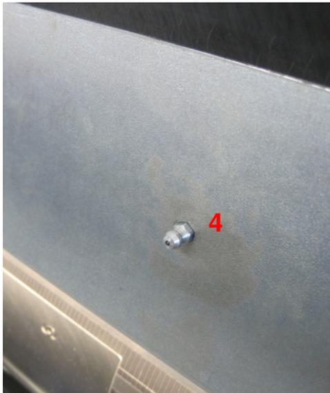
Figure 16: Maintenance point, pressure rollers
