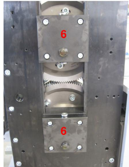
Figure 17: Maintenance point, magnetic cylinder bearing
