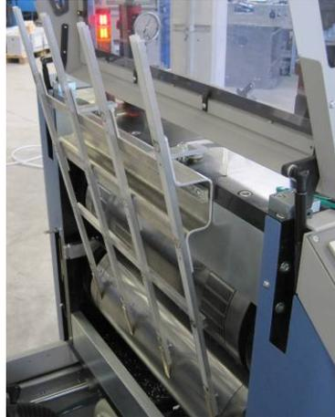
Figure 112: Punching sheet assembly aid
