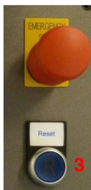
Figure 34: Emergency OFF with Reset button
