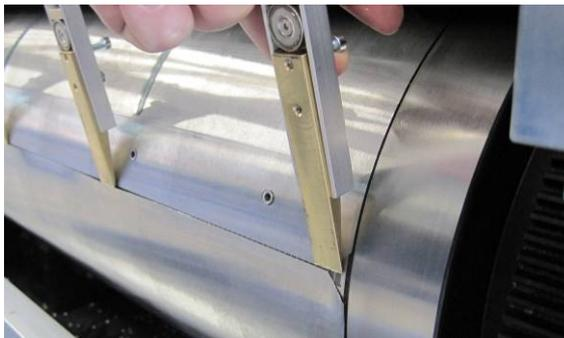
Figure 116: Magnet cylinder with feeder
