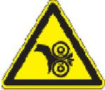
**Danger of rotating rollers.** Failure to comply may lead to serious personal injury and to material damage.
