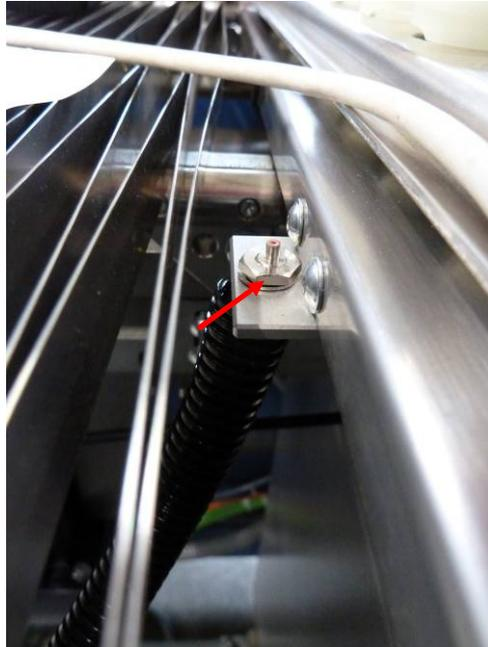
Figure 22: Optical sensor
