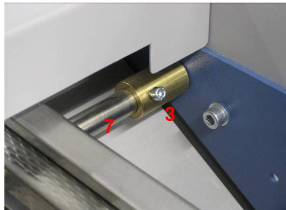
Figure 13: Loosening the screw
