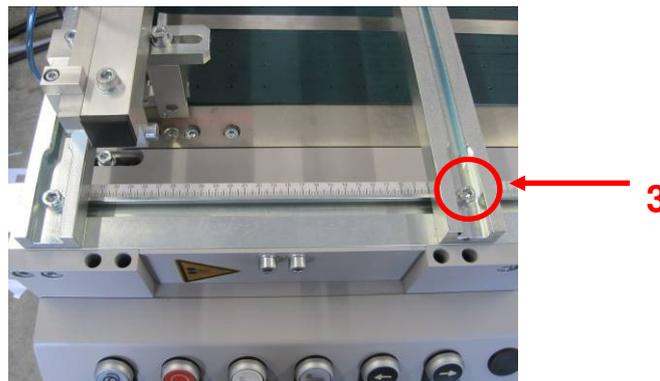
Figure 122: Belt carpet assembly bar
