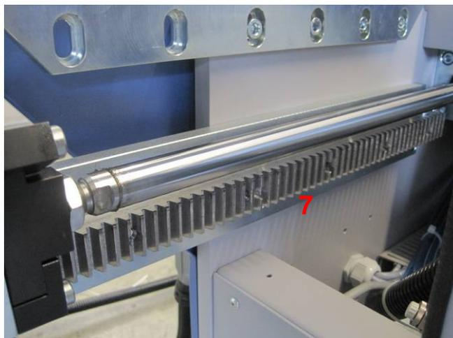
Figure 18: Maintenance point, runner rails
