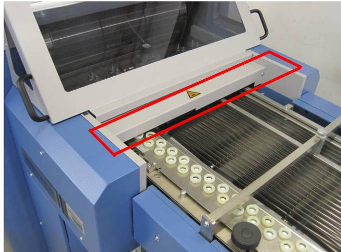
Figure 2: Hazard point, infeed
