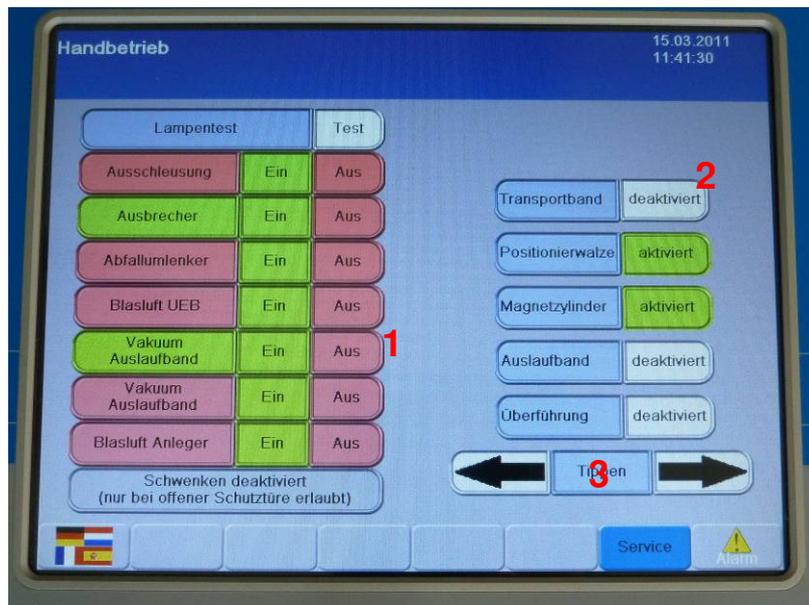
Figure 17: "Manual mode" display
