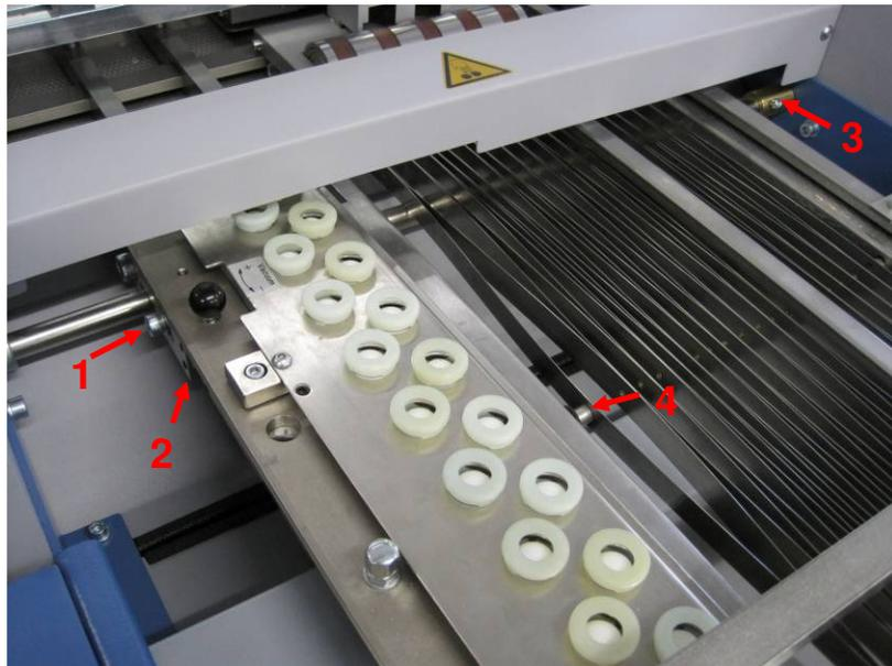
Figure 11: Changing the aligning belt
