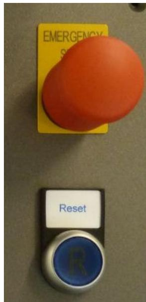
Figure 32: Emergency Stop with Reset button
