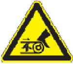
**Danger of rotating belt drive.** Failure to comply may lead to serious personal injury and to material damage.
