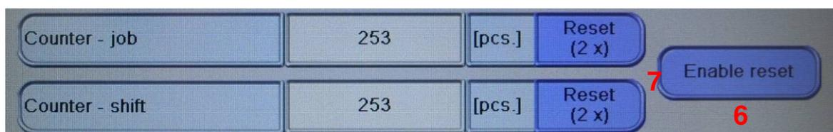
Figure 66: Reset of unit counters
