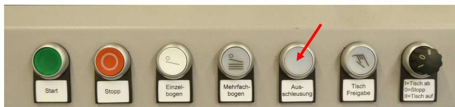
Figure 46: Eject buttons
