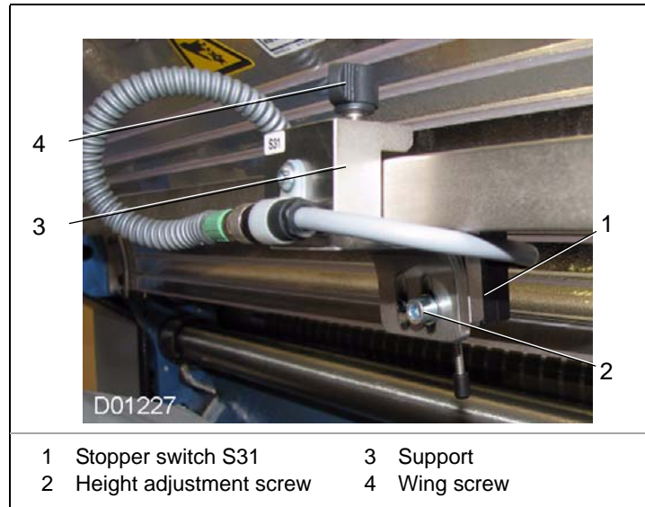
Figure 61: Stopper switch S31 at the exit of the folding unit
