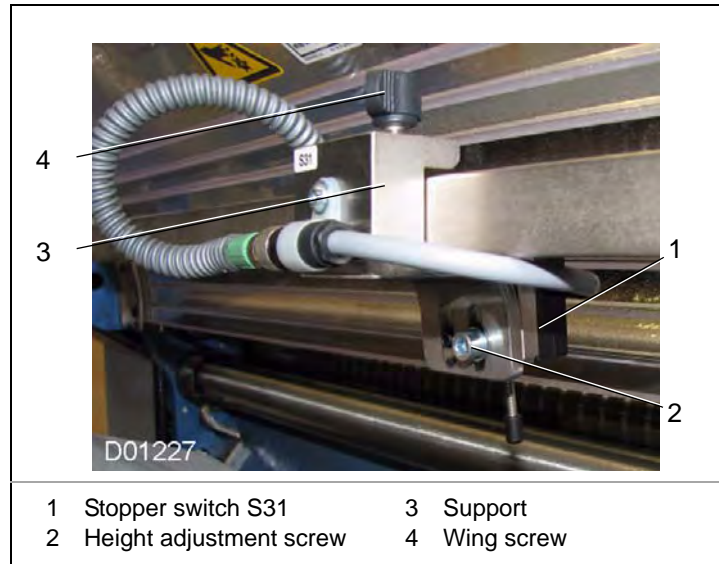
Figure 84: Stopper switch S31 at the exit of the folding unit
