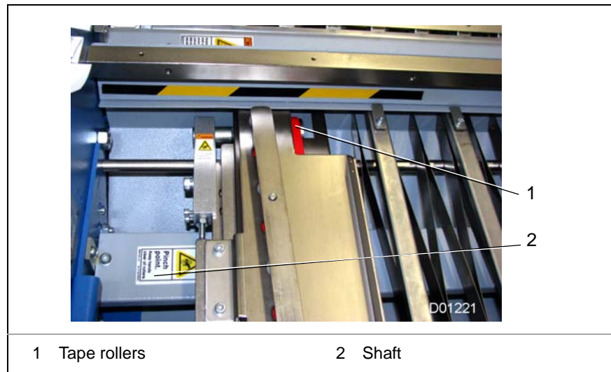
Figure 83: Hazard areas of the register table
