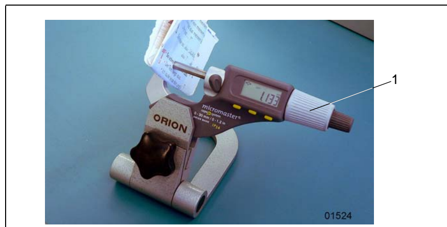
Figure 61: Measuring the paper thickness
