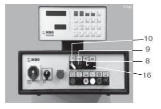
The pile plate **1** moves down and stops at a safety margin of approximately 15 cm above the floor. Push the button **16** continuously for further down movement.
