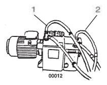
>ATTENTION< Check the clockwise rotation prior to initial operation! If the motor is turning counter-clockwise it may cause considerable damage to the pressure/vacuum pump!
