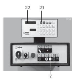
A "learning sheet" is passing the machine. The photocells detect lengths and times of passage. This will automatically program sheet control and sheet monitoring.
