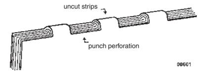
When using the new punch-perforation device, it is of the utmost importance that the punched out pieces are separated and stripped from the folded sheets. A new design of perforating knife ensures this in conjunction with a specially manufactured stripping unit.
