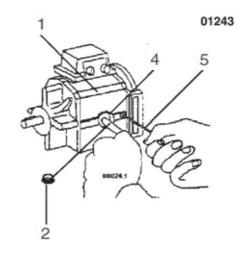
Retension counter nuts **3**. Make sure that screws are not distorted! Replace dummy plug **2**.
