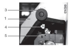
The switch 6 will stop the machine if the hood 1 is being opened.
