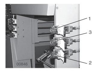
Slitter shaft at crossfold section 4 (quickly removeable through plug bearings)
