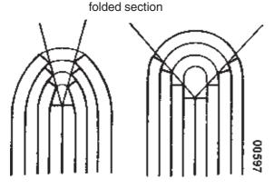
These slots provide a larger opening in the spine of the collated sections and allow the glue to penetrate easily and reach every single sheet.
