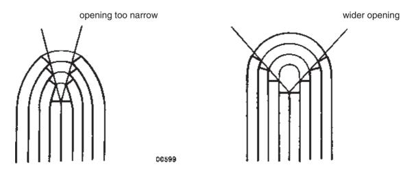
With punch-perforation the opening is larger and the angle wider, therefore the glue can definitely reach all sheets.
