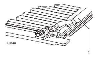
Heavy or multiple folded sheets may require an increase of the folding space **2**, for this purpose remove the deflector a little bit.
