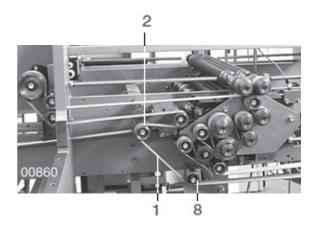
Re-tension the Poly-V belt **4** and remove the screws **6**, rotate the flange **7** and re-thread the tape **1**.
