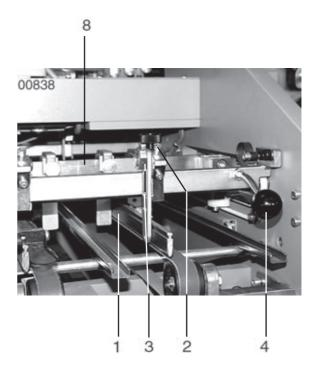
If crossfold sheet stop 8 is not used lift it up and turn OFF corresponding knife coupling for crossfold section. Turn toggle switch 9 into middle position.
