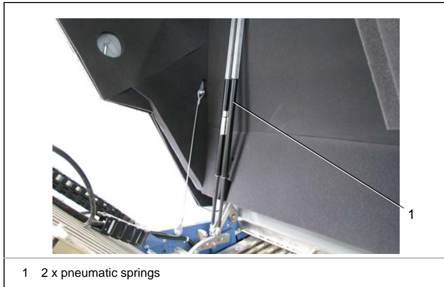
Illustration 195: Pneumatic springs on the noise damping and safety hood
