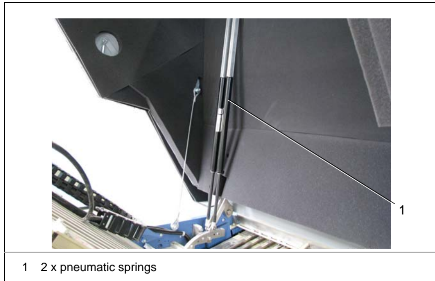
Figure 199: Pneumatic springs on the noise damping safety hood
