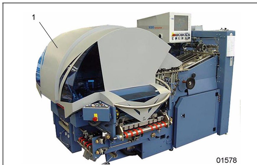
Figure 13: Safety and noise damping hood
