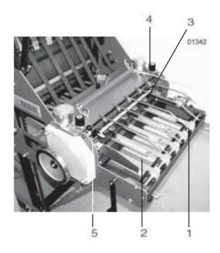
If a product that is too thick reaches this element the machine will be disconnected by the micro switch 5 to avoid a stoppage in the main pressing rollers 6.
