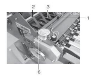
For this purpose swivel the lower tapes **3** over the stop bolt **4**.
