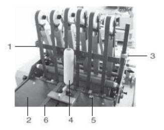
The speed of the transportation tapes 6 can be altered through the knurled nut 7.
