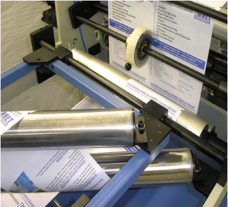
Fig.5.4.2 Entry and centre piece of Split & Merge Station
